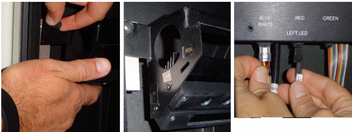
Figure 3.17. Remounting LED assembly and reattaching connectors
