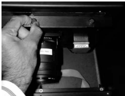
Open filter wheel access panel and rotate it downward
