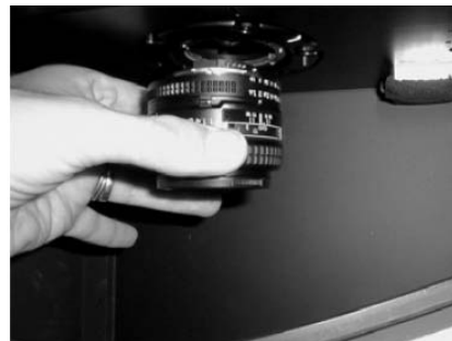
Figure 3.24. Steps in lens removal.
