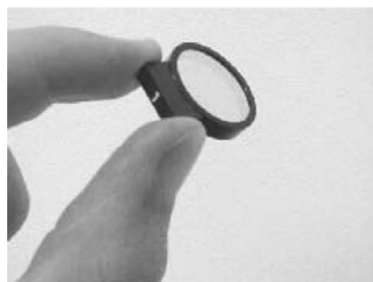
Figure 3.21. Unpack and carefully install filter 1. Make sure that filter 1 is all the way in its slot and positioned straight.
