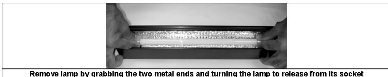
Figure 5.4. Removing epi-module lamp.
