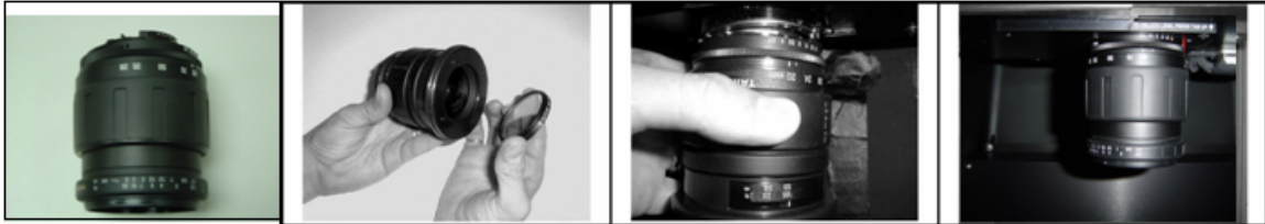
Figure 3.22. Steps in zoom lens installation
