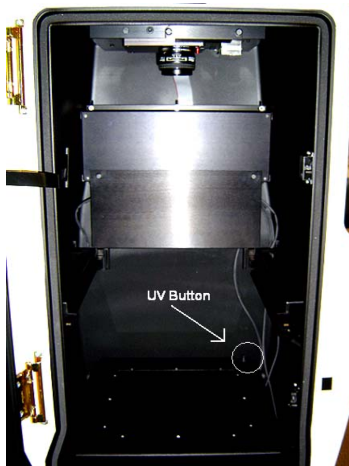
Fig. 4.3 VersaDoc sample platen UV button
