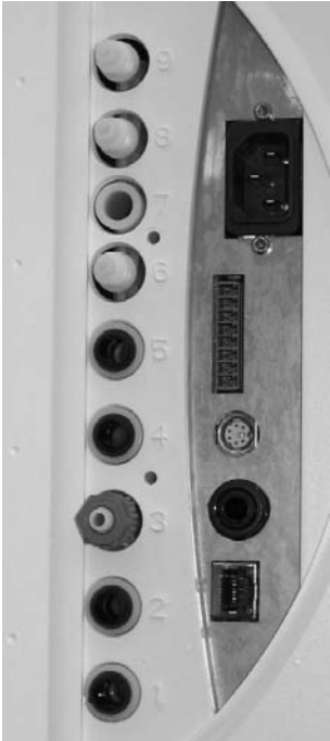
RC-Link tubing to Port 4.
