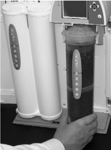
Top of Quantum Cartridge being pushed into place
