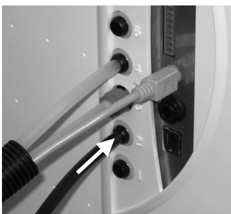
Feedwater tubing attached to Port Number 2.
