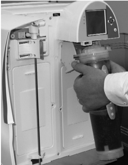
Quantum Cartridge being pulled out from the pack adapter.
