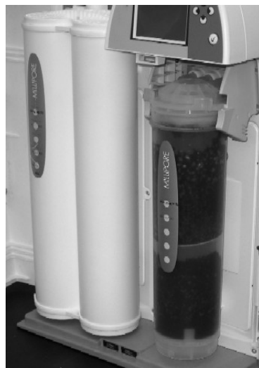
Quantum Cartridge installed.
