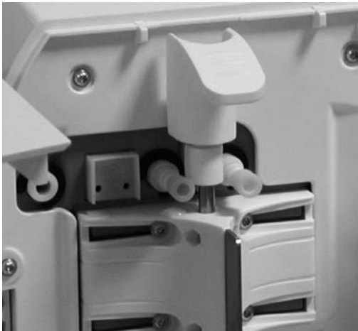
Pak Locking Handle lifted up.
