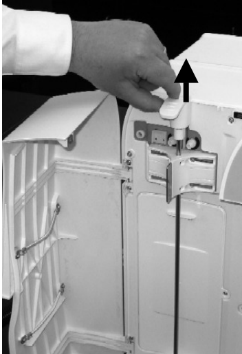
Q-Gard Pack pushed in at the bottom.
