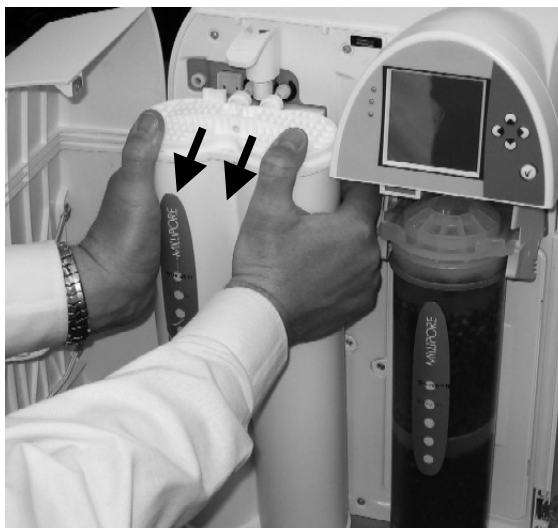
Q-Gard Pack being pulled out.
