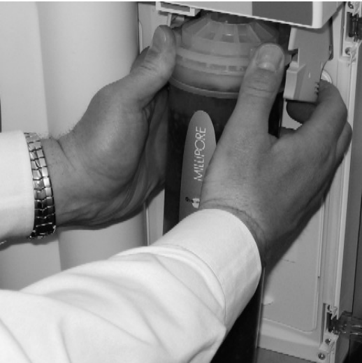
Quantum Cartridge installed.
