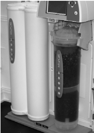
Quantum Cartridge installed.
