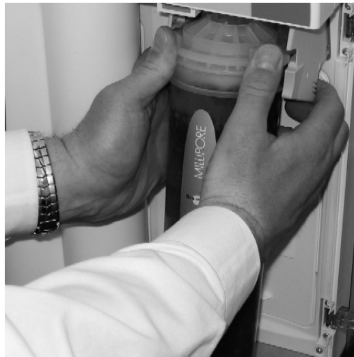
Quantum Cartridge installed.
