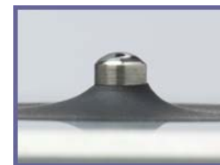
Un-conditioned Pedestal- water “Flattens out”
