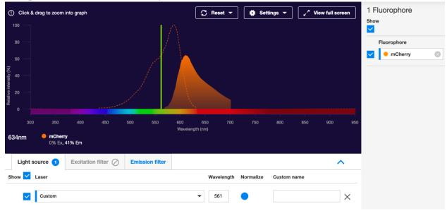
**Step 3:** Ensure the emission filters capture the emission spectra of your fluorophores.
