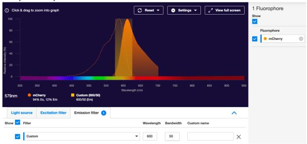
**Step 4:** If using multiple fluorophores ensure they can be sufficiently separated. Example of good separation vs non separation:
