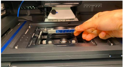
4. Position the sample in the path of the objective.
