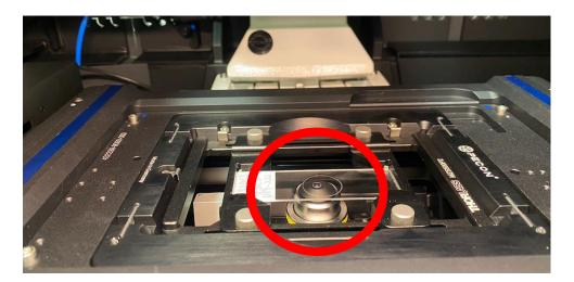
6. Choose the most abundant and brightest fluorophore to find focus, e.g. DAPI nuclear stain. Put DAPI cube in the light path, open the light source shutter, and direct light to the eyeyepiece
