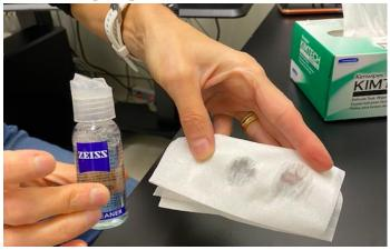
**Step 3**) Begin cleaning the sample/objective using the preparedkimwipe. Start in the center and work your way outwards in a circular motion.
