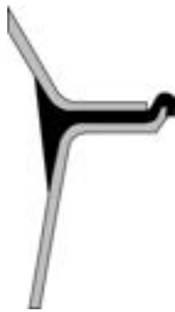
Lid Seal Cross Section
